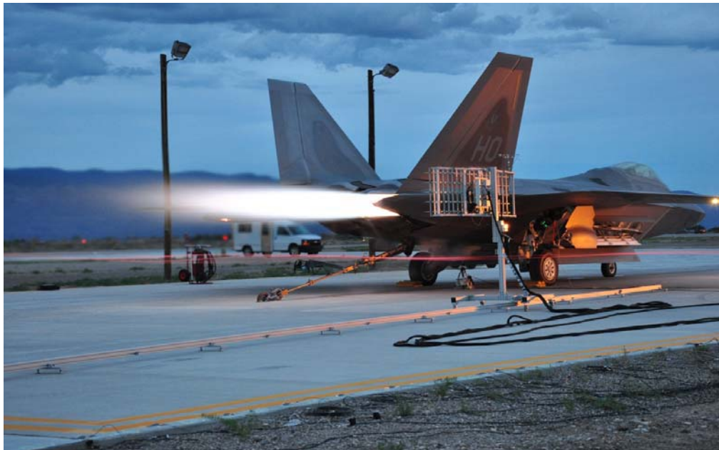
FIGURE . F-22 engine firing with measurement array and intensity probe shown. The intensity probe is positioned on top of the array, on the far right.
