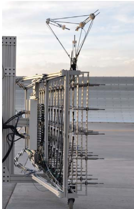
FIGURE 2. Close-up of intensity probe atop the microphone array. The probe microphones were mounted at the vertices of the external frame, pointing inward and located 1.9 cm from the geometric center.
