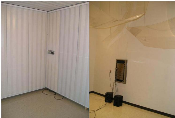
Figure 4. Left: variable acoustics room. Right: One of two coupled reverberation chambers
