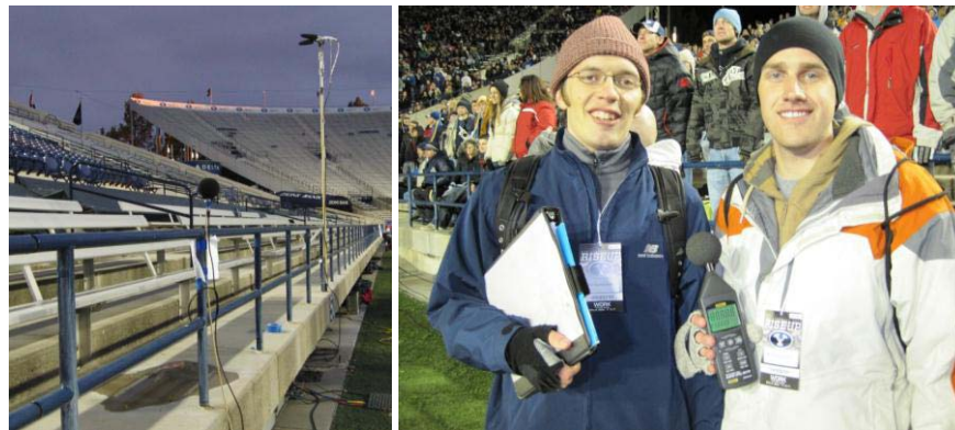
FIGURE 2. Left: Sideline microphone attached to railing and encased in a spherical foam windscreens. Right: A student team with logging Class-1 sound level meter and logbook.
