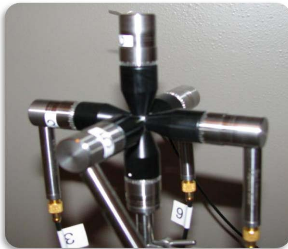
FIGURE 2. A six-microphone energy density probe. This probe enables two plane's of measurements to be made simultaneously while using four mid-plane microphones to estimate the gradient on these two planes.
