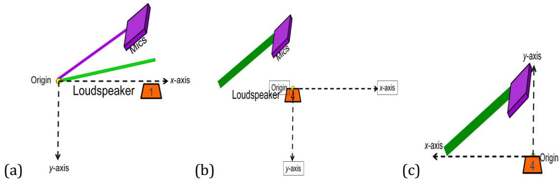
**Figure 7** (a) The data used for the conical NAH is measured at an angle of 30 degrees with respect to the origin that is 1 m from loudspeaker 1. (b) The coordinate system is translated in the x-direction so the loudspeaker is at the origin. (c) The coordinate system is rotated 180 degrees about the z-axis, such that microphones on the lower half of 8x8 array (represented by the purple box) are in the first quadrant.
