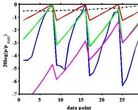
**Figure 6** The 10-degree data on 29 microphones at 1700 Hz (blue) is compared to the reconstruction results, based on the origin shown in Fig. 7(a), for conical NAH with  $N=0$  (red), 1 (green), 2 (black), 3 (magenta).
