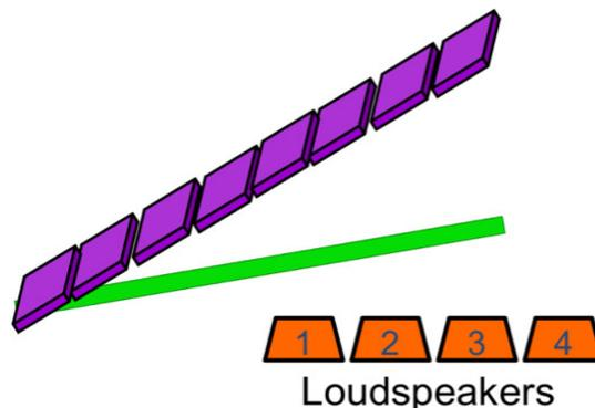
Figure 5 Drawing of the experimental set-up. The pressure from the loudspeakers is recorded on an  $8 \times 8$  microphone array at various positions along an angle of 30 degrees (purple) and 10 degrees (green) relative to the face of the loudspeakers.
