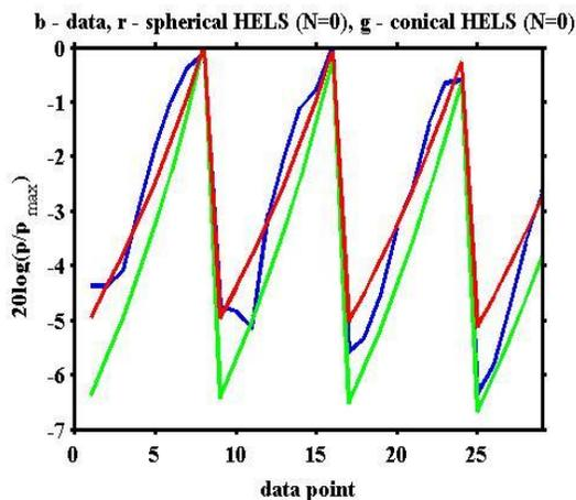
**Figure 8** Reconstruction results of conical NAH compared to the data recorded on 29 microphones at a frequency of 1700 Hz (blue) when the approximate origin is used (green) and when the optimal origin is used (red).  $N=0$  was used for these monopole reconstructions.
