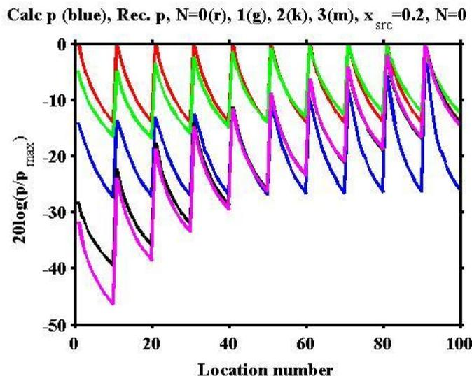
Figure 4 Calculated pressure field (blue) for a monopole at  $x=0.2$  compared to the reconstruction results with  $N=0$  (red), 1 (green), 2 (black), and 3 (magenta) in conical HELS.
