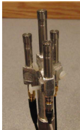
Figure 11. Four 6.35 mm microphones mounted in a regular tetrahedral arrangement.
