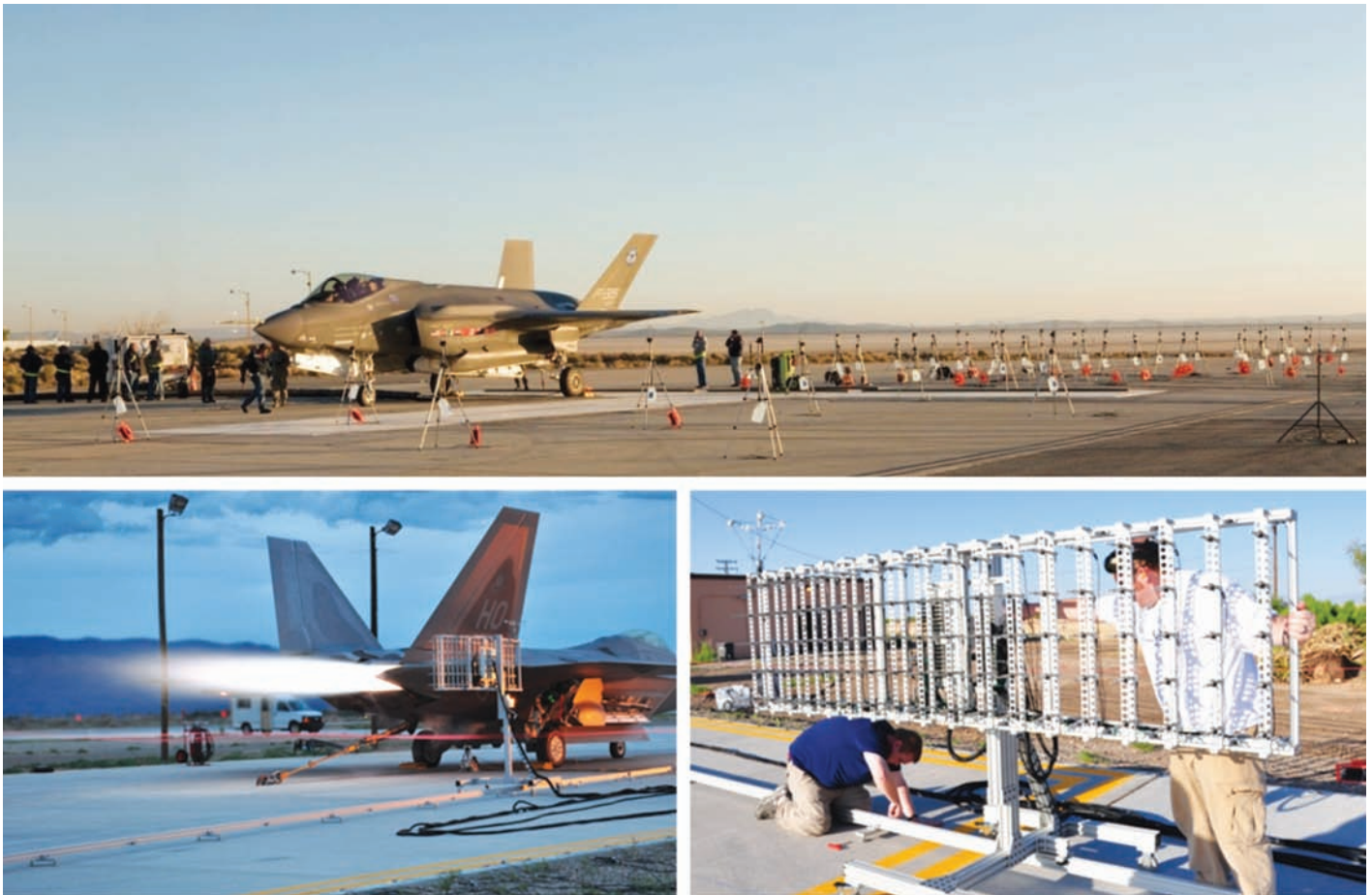
Fig. 6. Top: 2008 F-35AA Joint Strike Fighter measurements at Edwards AFB. The microphones were located on thin rods attached to the top of the tripods. Bottom: Near-field measurements of the F-22A Raptor at Holloman AFB in 2009. The measurements consisted of a ground-based linear array of microphones and a rectangular 90-microphone near-field acoustical holography array.
