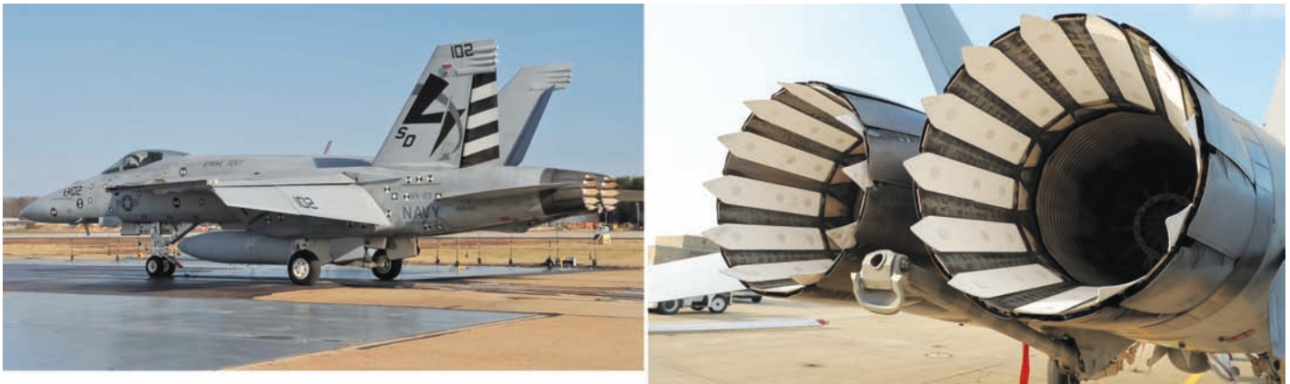
Fig. 3. Chevrons installed in the engine nozzles of an F/A-18E/F Super Hornet. Courtesy of the U.S. Naval Air Systems Command (NAVAIR).
