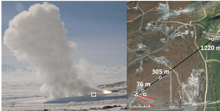
Fig. 1 (Color online). Picture of a GEM-60 SRM static firing and an annotated Google Earth ® satellite image of the ATK test area. The triangle shows the location of the origin, and the circles show the locations of the three microphones along the radial 60^\circ relative to the downstream direction. A sense of scale is provided by the picture and the map, both denoting the location of a large rock pile about 95 m from the rocket nozzle.
