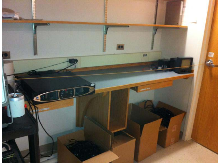
FIGURE 1. General experimental configuration used. The vibration shaker can be seen on the left, with the power amplifier located behind. The string is stretched from the shaker over to a doorknob, with it simply being tied at both ends. The signal generator is located just to the left of this picture.
