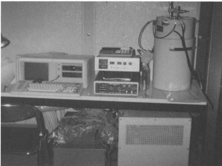
Figure 1a. Photograph of detector (right) holding two sample cylinders, also two JSR-11 analyzers (see text) and portable PC for data acquisition. (Set-up in Kamioka, Japan).
