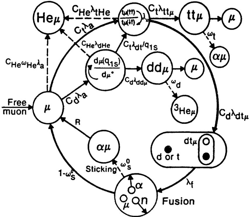
Figure 2. Scheme of the muon-catalyzed fusion cycle, showing reactions which occur when negative muons stop in a mixture of the hydrogen isotopes (p, d, and t) and helium (He) with respective fractions  $C_p$ ,  $C_d$ ,  $C_t$ , and  $C_{He}$ . Reaction rates are labeled with  $\lambda$ , and muon loss probabilities are labeled with  $\omega$ .
