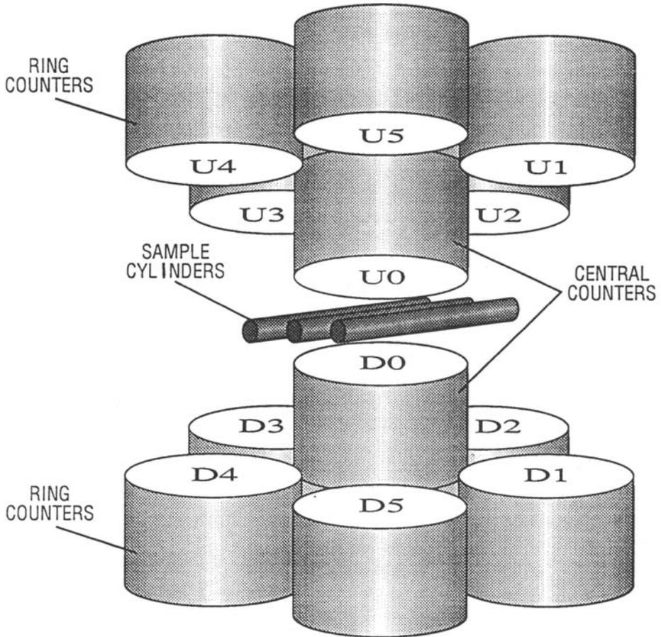
Figure 1. Schematic view of the Yale experiment (August 1989) indicating relative positions of central and ring counters. Liquid-scintillator filled counters were actually five-sided and about 17 cm deep; light guides also had sharp angles. Pulse-shape discrimination was used to help distinguish neutrons from gammas (see Table I).
