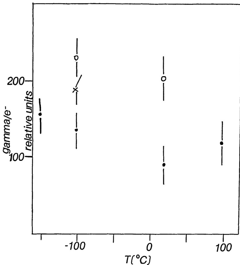
Figure 2: Relative yields of fusion gamma ray/muon decay electrons (arbitrary units). Open circles 0, 83%  $H_2$  + 17%  $D_2$ ; X, equilibrated mix from above, 56%  $H_2$  + 38%  $HD$  + 6%  $D_2$ ; closed circles 0, 48%  $H_2$  + 52%  $HD$
