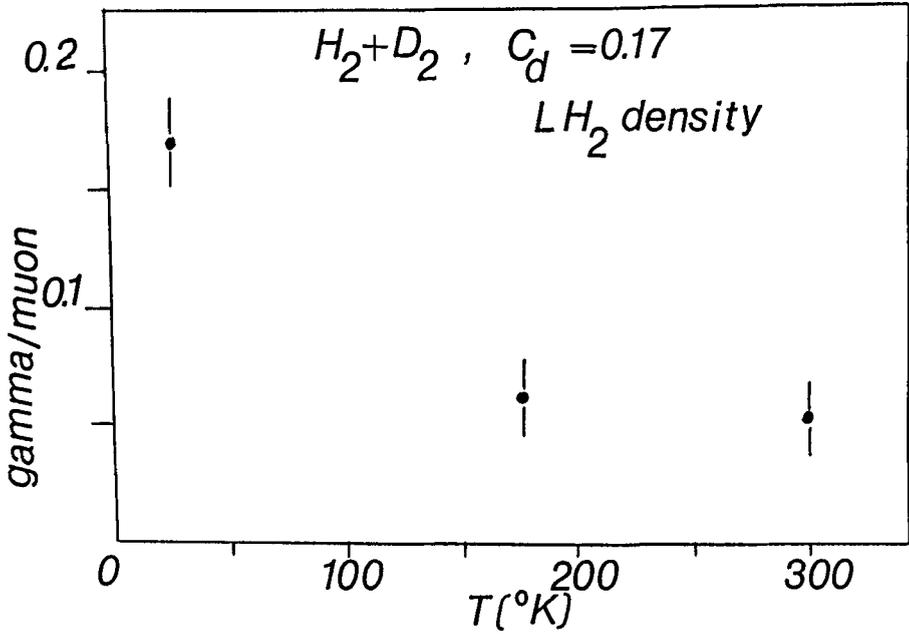
Figure 3: Absolute yield of fusion gamma rays per muon. The points at 173°K and 300° are our new data normalized to liquid hydrogen density using  $\lambda_d(\frac{3}{2} \rightarrow \frac{1}{2}) = 42 \times 10^6 \text{ s}^{-1}$ . The point at 22°K is scaled value of ref. (6) for a 17% deuterium concentration.
