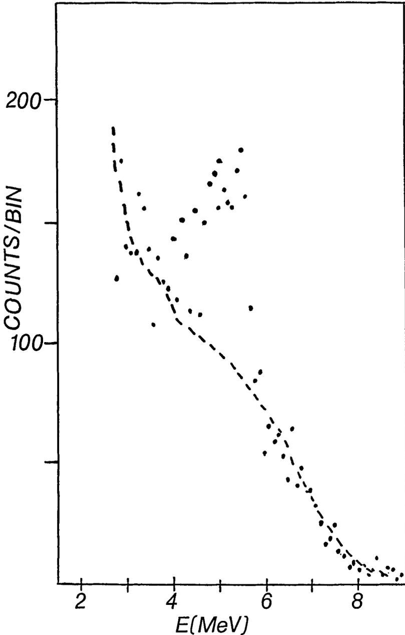
Figure 1: Gamma ray spectrum (dotted) from the  $H_2 + D_2 = C(D_2) = 0.17$  target. The background spectrum is shown as the dashed line. The bin size is 0.1 MeV. The gamma ray from the  $p + d \rightarrow {}^3\text{He} + \gamma$  reaction is visible.
