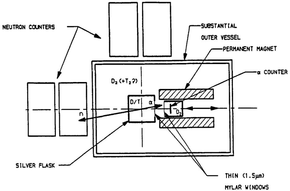
Fig. 1. Apparatus for measuring  $W_s$ .
