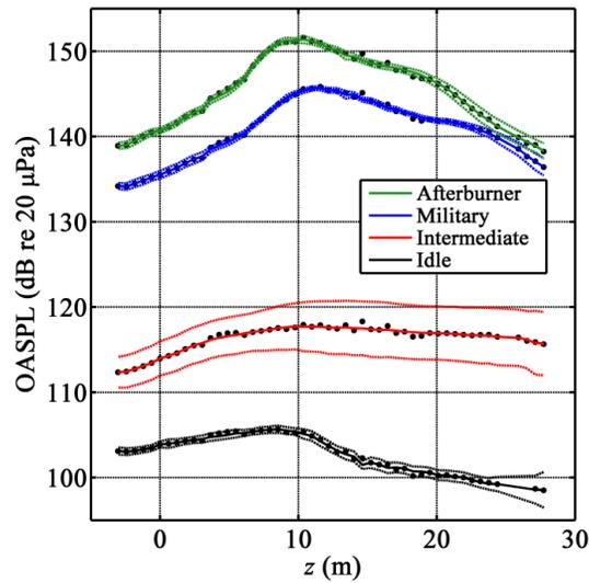
Fig. 3 - OASPLs measured along the ground 12.0 m from the jet centerline by the reference array, for all engine power conditions. Black dots indicate averages of directly measured values and exhibit slight spatial noise due to microphone-sensitivity biases. Smoothed data are shown by a solid colored line, and  $\pm 1$  standard deviation over all scans is represented by colored dashed lines.
