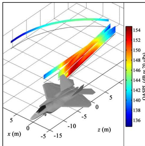
Fig. 2 - OASPLs measured in the geometric near field at afterburner engine conditions. Levels are plotted at their three-dimensional locations.
