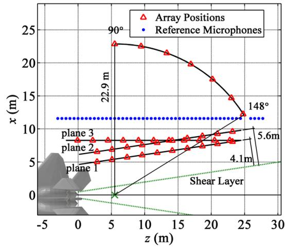
Fig. 1 - Schematic of the measurement locations, relative to the aircraft. The estimated shear layer boundary is marked by green dashed lines, and the green "x" delineates the estimated maximum-noise-source region and the center of the arc.
