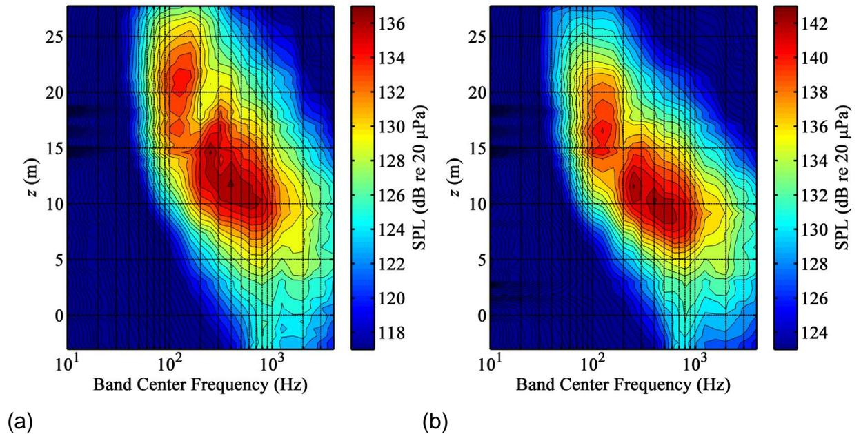
Fig. 6 – One-third octave spectral variation over location along reference array at (a) military and (b) afterburner engine conditions. Each contour line represents a step size of 1dB.
