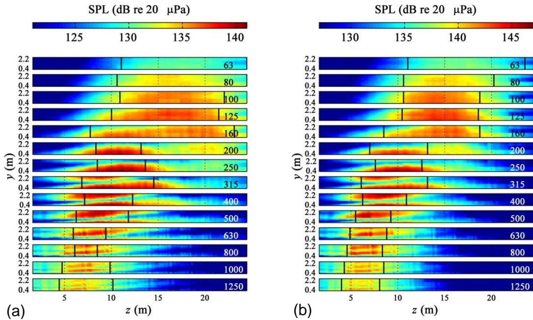
Fig. 5 - SPLs measured at plane 2 for several one-third octave bands at (a) military and (b) afterburner engine power conditions. Vertical black lines indicate the regions where SPLs are within 3 dB of the maximum SPL. The number at the right of each plot is the band center frequency in Hz.
