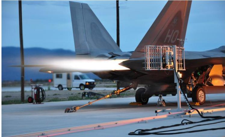
Fig. 1 -The F22A Raptor tied down to the run-up pad with the 90-microphone array shown.
