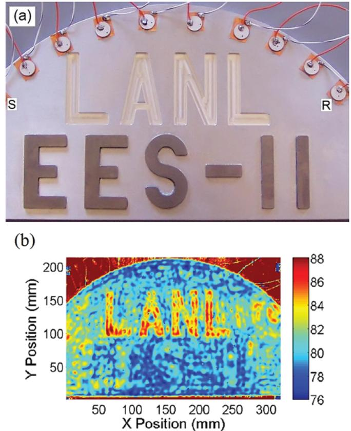
Fig. 2. (a) Photograph of a semicircular aluminum plate which has the letters "LANL" milled out of it and steel letters "EES-11" glued onto it<sup>15</sup>. S and R denote the source and receiver transducers named according to the forward propagation usage. (b) RTM image of the other side of this plate (mirror image is displayed). Amplitude is in dB units with an arbitrary reference.
