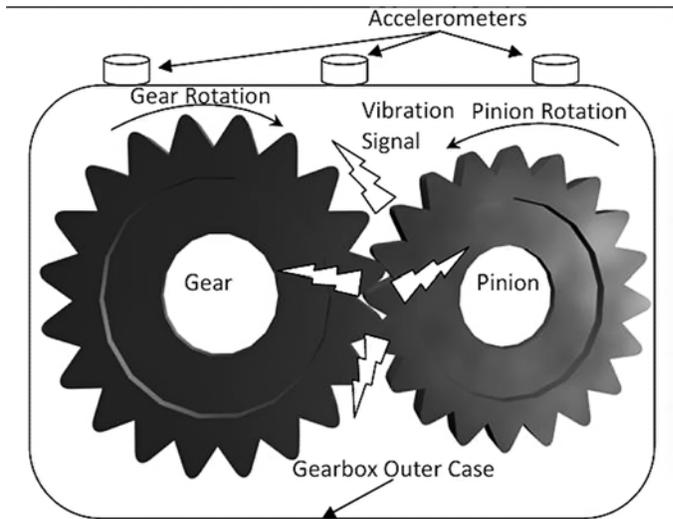
Fig. 3. Simple spur gear and pinion setup.
