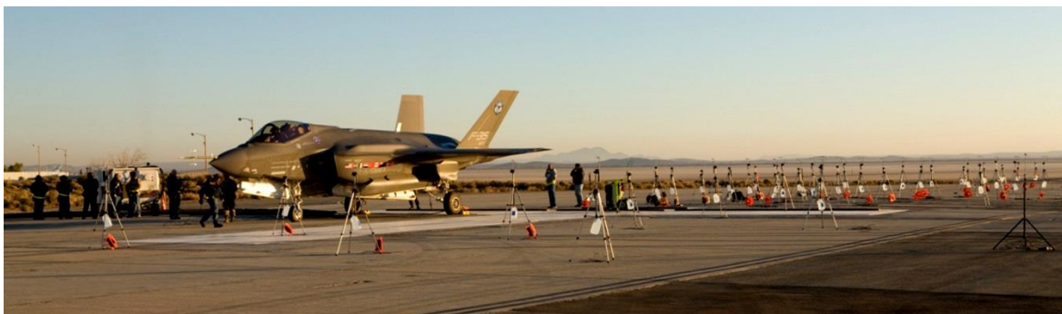
Figure 1. Tied-down F-35AA aircraft, along with tripods of the near-field microphone array.
