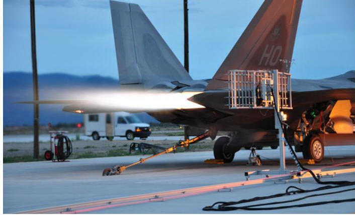
Figure 2. The tied-down F22A Raptor with one engine at afterburner. Shown also is the 90-microphone rectangular array.
