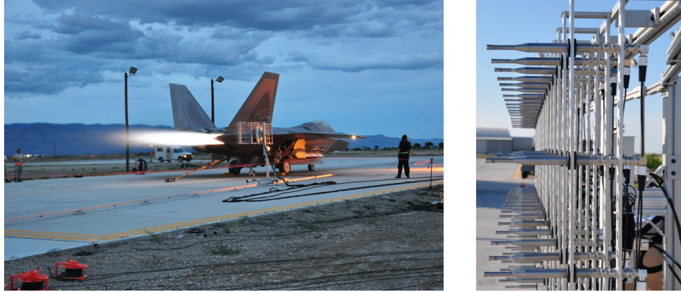
Figure 2. Photographs from F-22A test in 2009. The rectangular array of microphones with guide rail is shown near the aircraft. The ground-based microphone array is located just inside the edge of the pavement. A close up of the array is shown on the right.
