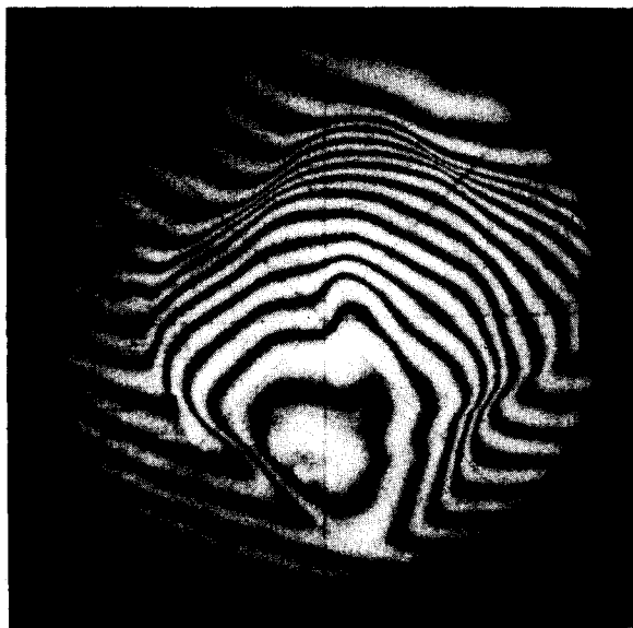
FIG. 3. An end-on hologram of the plasma in FRX-C is displayed. 3 The external multipole field is oriented as in Fig. 1.
