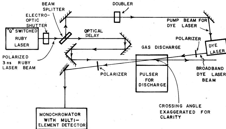
FIG. 6. Schematic diagram of the proposed experiment to detect stimulated Thomson scattering.
