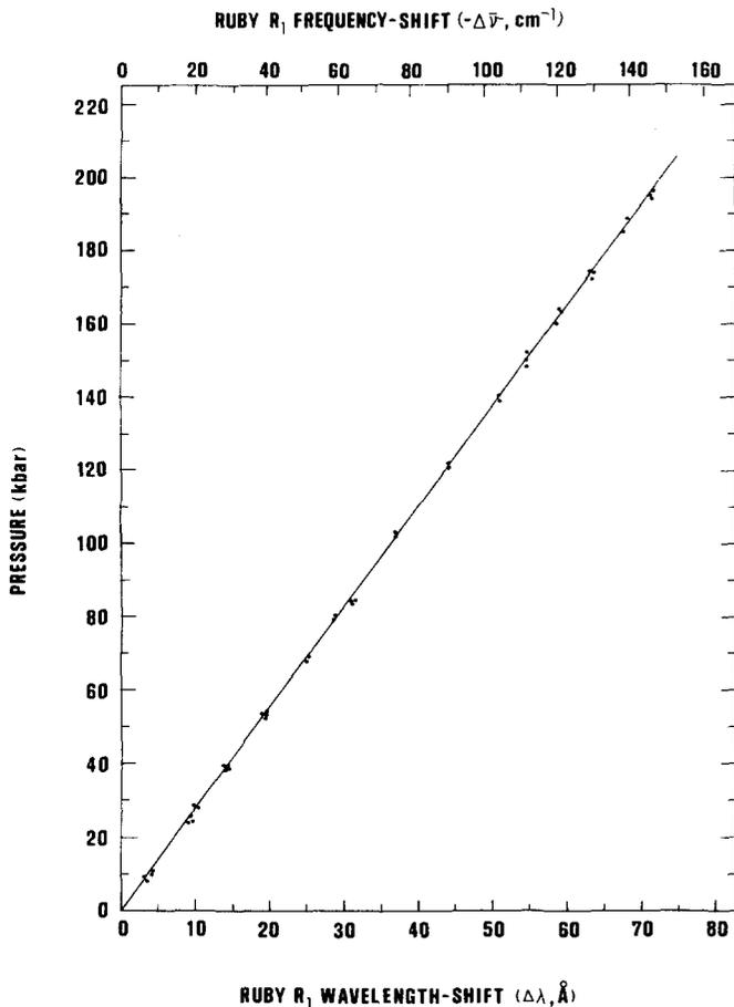
FIG. 1. The pressure dependence at 25°C of the ruby  $R_1$  fluorescence line at 6942 Å as a function of wavelength (Å) and also wave number or frequency ( $\text{cm}^{-1}$ ). Pressure values are based on the Decker equation of state for NaCl.
