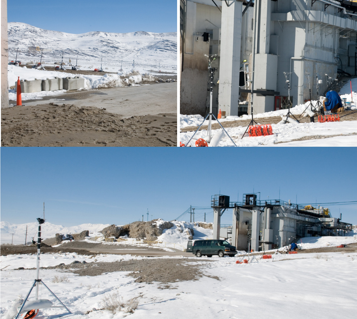
Figure 4. Photographs of near-field array during the 2-19-09 test setup. Top Left: View from near nozzle showing terrain variation. Top Right: View of the test bay shot from near the farthest external frame tetrahedral probe ( 35D downstream of the nozzle exit). Bottom: View of the test bay from just beyond the farthest near-field microphone ( 50D downstream of the nozzle exit). Cables from the array were run uphill to the rear of the test bay, where the recorder was located.
