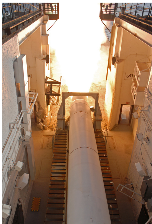
Figure 6. Photograph of the 2-19-09 GEM-60 static firing from inside the test bay.
