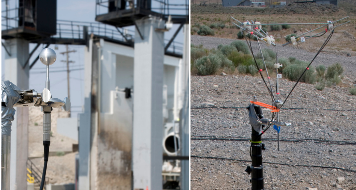
Figure 1. Left: spherical probe with GEM-60 test bay and nozzle in the background. Right: External frame tetrahedral probe utilizing four matched condenser microphones. This probe is an inverted tetrahedron, where microphone 1 is beneath the horizontal plane containing microphones 2, 3, and 4.
