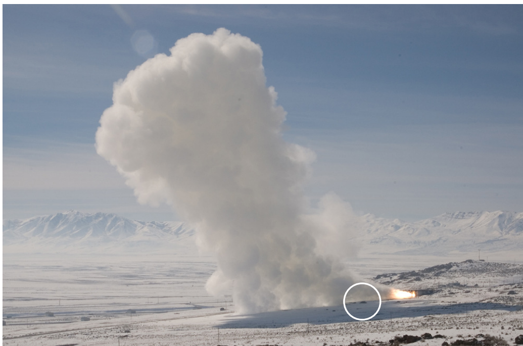
Figure 7. Photograph near the end of the 2-19-09 static firing, where the length of the visible flame is considerably shorter than at the beginning of the test. Circled is a cluster of rocks that were approximately 55D downstream of the nozzle. The 50D microphone pictured at the bottom of Fig. 4 was near these rocks.
