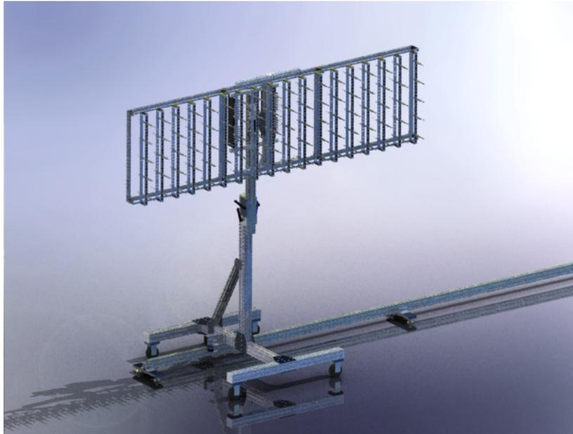
Figure 4. Conceptual image of the test rig structure positioned with the microphone array in its highest horizontal configuration.
