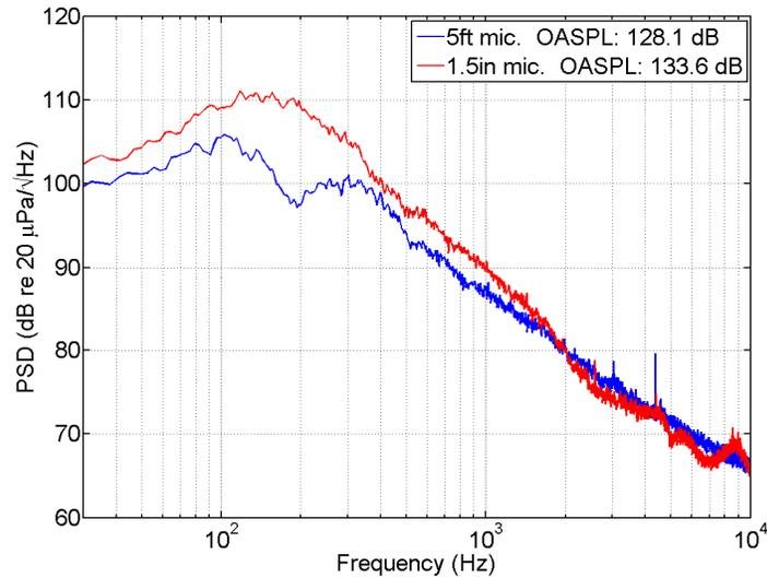
Figure 3. Comparison of spectra measured at the same downstream and lateral position, at heights of 5 feet (1.5 m) and 1.5 inches (0.038 m).
