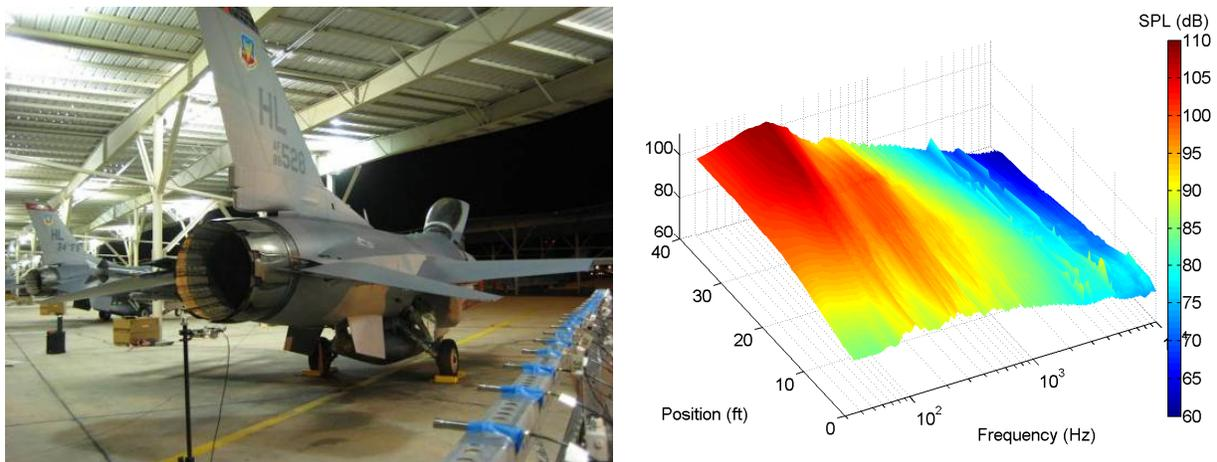
Figure 2. F-16C microphone array on left, SPL map of plume on right.
