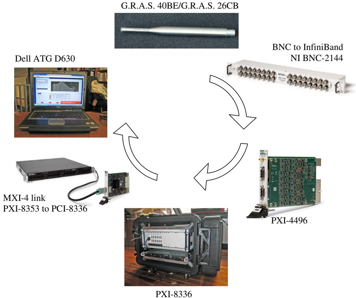
Figure 6. Measurement instrument chain from microphone to hard drives.
