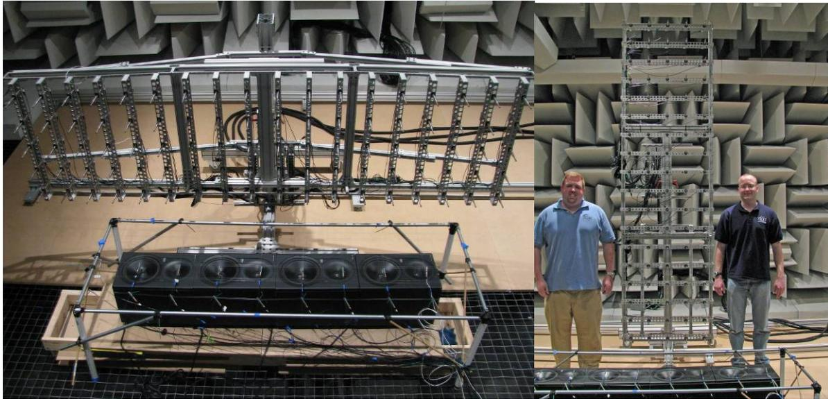
Figure 5. NAH measurement system pictured in horizontal configuration on left, and vertical configuration on right.
