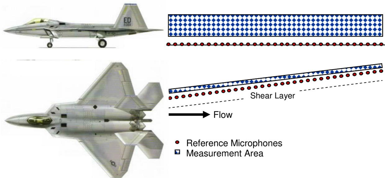
Figure 1. Plan and top view schematic of jet plume acoustic measurement area of interest.
