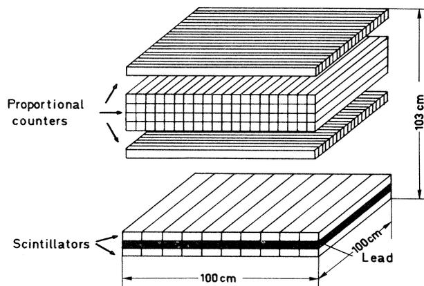
FIG. 1. Schematic view of hodoscope and scintillators.
