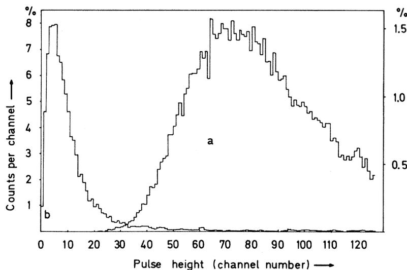
FIG. 2. Measured pulse height distributions for (a) particles of unit charge and (b) quarks. The distribution for quarks was simulated by observing particles of unit charge in counters built to  $\frac{1}{3}$  scale.
