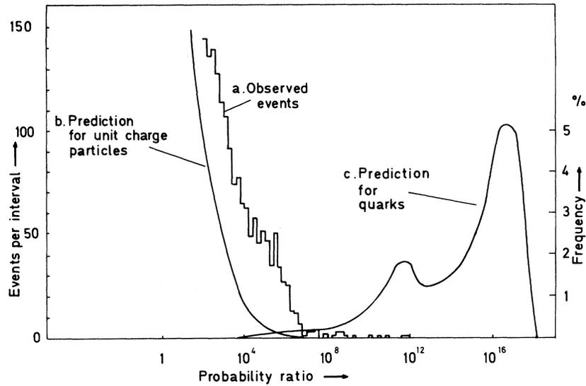
FIG. 3. Distributions of probability ratios: (a) tail of observed distribution, (b) Monte Carlo prediction for unit-charge particles normalized to the total number of particles observed, and (c) Monte Carlo expectation for quarks.
