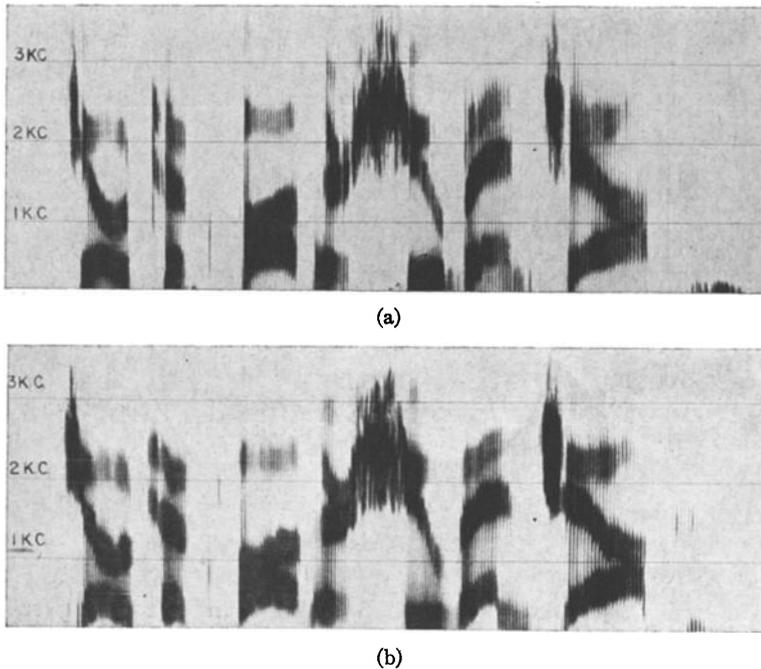
FIG. 9. Spectrograms of "Joe took father's shoe bench out." Upper: Natural. Lower: Synthetic.
