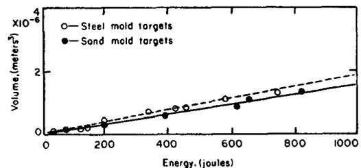
FIG. 9. Crater volume vs pellet energy for the alloy of 30% lead and 70% tin.
