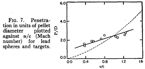
FIG. 7. Penetration in units of pellet diameter plotted against  $u/c$  (Mach number) for lead spheres and targets.
