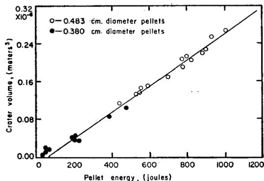
FIG. 3. Relationship between crater volume and pellet energy when mild steel (1040) spheres are fired into semi-infinite targets of the same composition.
