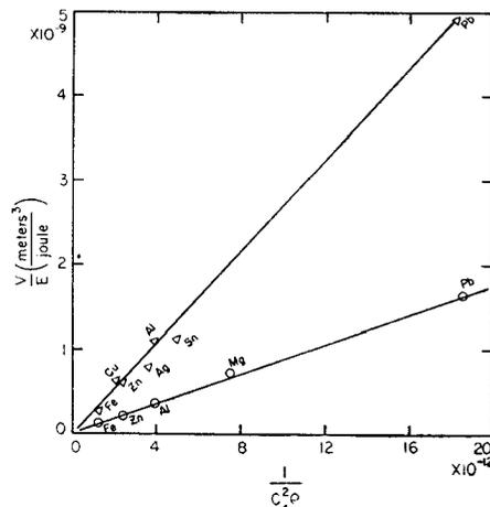
FIG. 5. Volume per unit energy plotted against the parameter,  $1/c^2\rho$ , for several pure metals.
