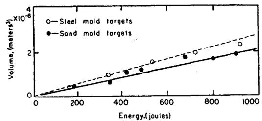
FIG. 8. Crater volume vs pellet energy plotted for the alloy of 80% lead and 20% tin.
