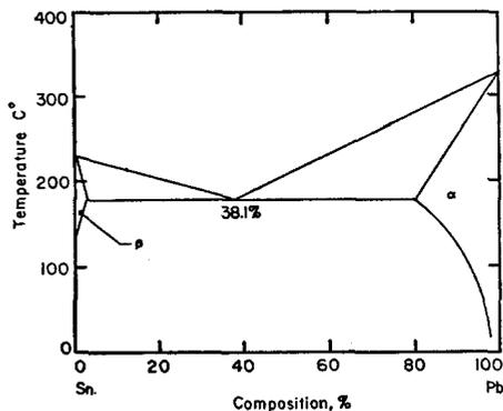
FIG. 11. Phase diagram for the lead-tin alloy system.
