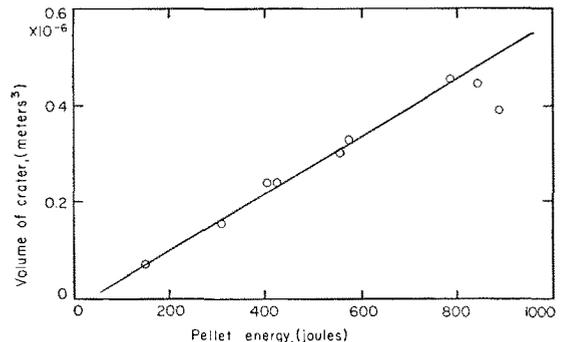
FIG. 2. Relationship between crater volume and pellet energy when zinc spheres are fired into semi-infinite zinc targets.
