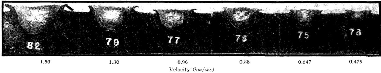
FIG. 1. Photograph of a series of sectioned craters formed in a lead target by 0.483-cm diameter lead spheres. Impact velocities are indicated for each crater.
