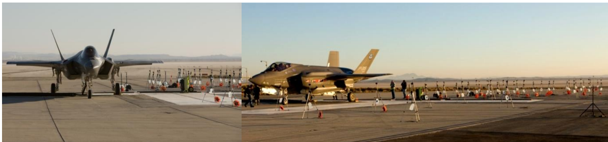
Figure 1. Tied-down F-35AA aircraft, along with tripods of the near-field microphone array.
