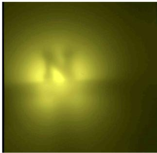
**FIGURE 1.** Single-shot electron beam radiograph of a 1.27x1.27x3.8 cm deep stainless steel N-bar, shielded by 2.5 cm Al. The illuminated face of the N-bar distance was located 84 cm from beam source and 6 cm from image plate. Millimeter-scale features are clearly apparent. (The platform and stalk supporting the N-bar are also visible.)
