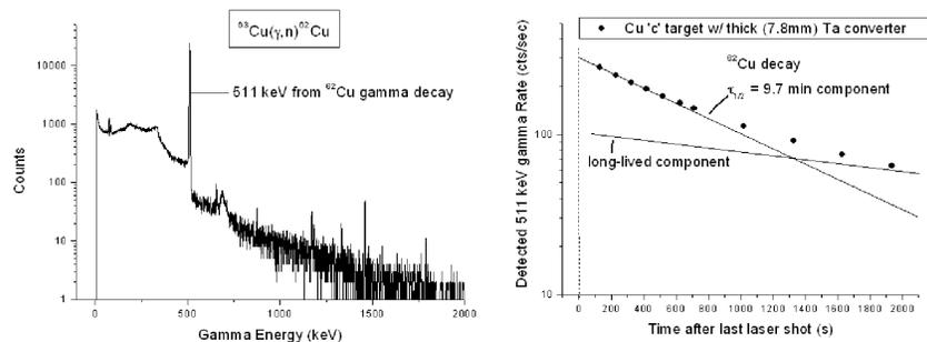
**FIGURE 2.** Measured spectrum from electron-beam-activated Cu target (left), and measured decay curve (right) exhibiting 9.7-minute half-life that identifies <sup>62</sup>Cu. This is the longest-standoff activation performed using a laser-based source. This test case demonstrates capabilities to be applied to shielded SNM.
