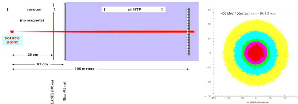
**FIGURE 3.** Simulation of 400 MeV electron transport through 100 m of air at STP. Left: geometry and material setup for radiography simulation. Right: GEANT Monte Carlo code calculation of normalized electron fluence at detection plane; contours indicate 0.17, 0.33, 0.5, 0.67, 0.83 of peak fluence. A large fraction of the beam remains undeflected or slightly deflected.
