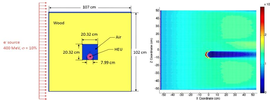
**FIGURE 4.** Simulation of 400 MeV electron transport and shower production in thick wooden crate containing highly enriched uranium (HEU). Left: simulated geometry; right, electron fluence (cm<sup>-2</sup>) throughout crate. Fluence grows after penetration into the crate, as incident electrons produce showers of lower-energy electrons. 8 cm HEU sphere casts a clear shadow through 0.5 m of wood.
