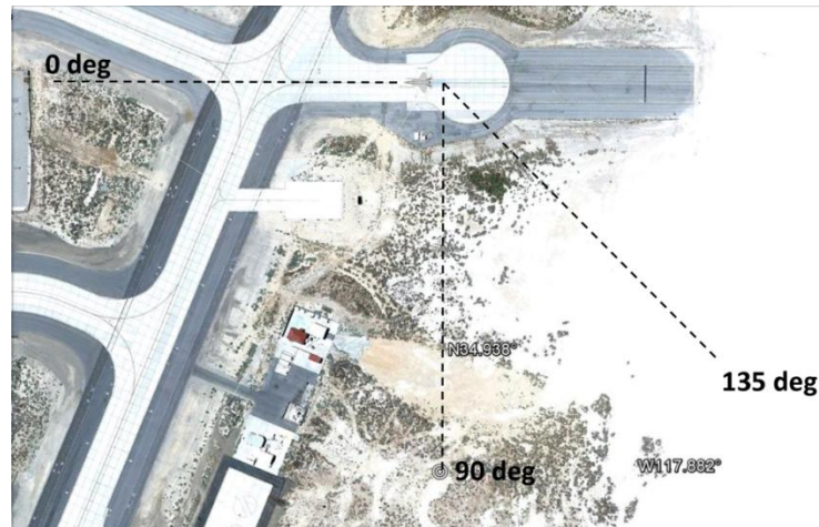
Figure 4. Run-up pad environment at Edwards Air Force Base. The radial lines are 305 m (1000 ft) in length; the origin is located 6.7 m downstream of the nozzle exit.
