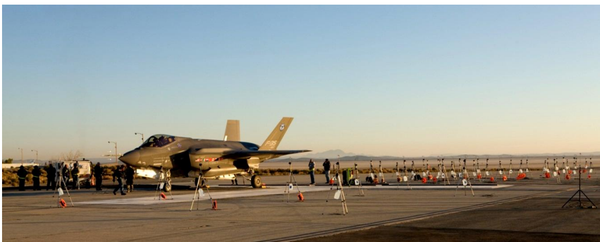
Figure 1. Tied-down F-35AA aircraft at Edwards Air Force Base. Also visible are some of the tripods of the near-field microphone array.
