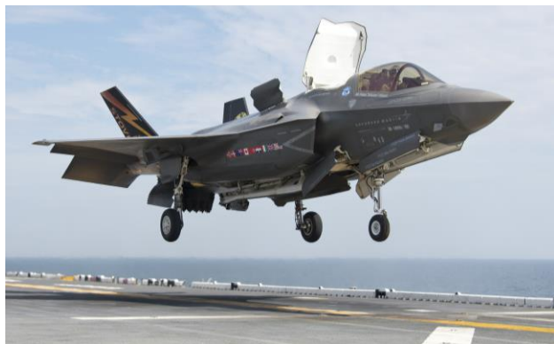
Figure 1. Vertical landing of an F-35B. An F-35B lands on aboard the USS Wasp during August 2013. In order to perform a vertical landing, the three-bearing swivel module rotates the engine exhaust nozzle to face downward and the LiftFan® operates near the front of the aircraft. Photograph in the public domain. 13
