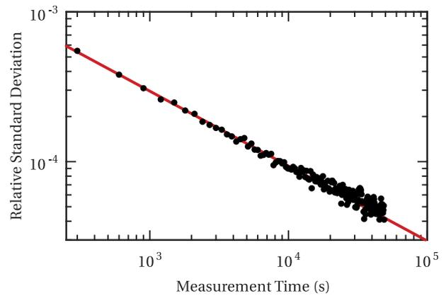
FIG. 3. Relative standard deviation of a NaI scintillator count rate as the measurement time is varied. The total count rate from the  $^{152}\text{Eu}$  sample, integrated over all energies, was measured on two detectors over a period of seventeen days. The solid line indicates that the uncertainty scales as the square-root of the measurement time, as expected.
