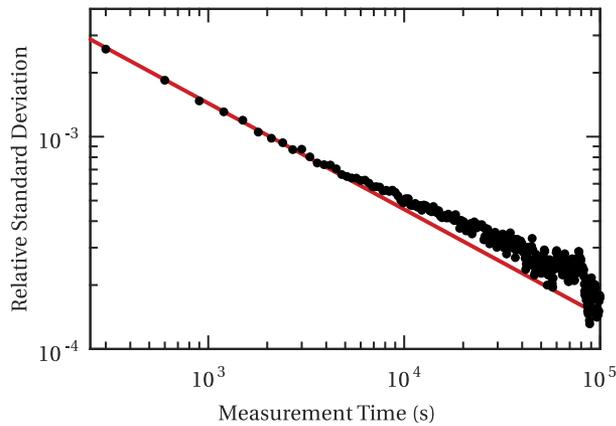
FIG. 2. The relative standard deviation of the GM count rate measurements for the  $^{36}\text{Cl}$  sample plotted versus the measurement time. The solid line indicates that the uncertainty scales as the square-root of the measurement time, as expected.
