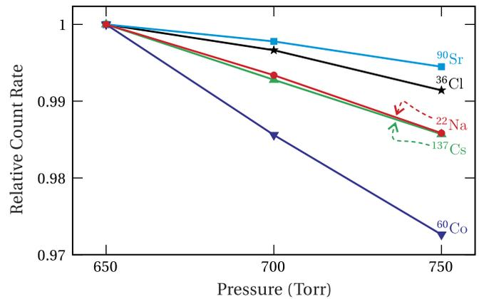
FIG. 5. Relative count rate versus pressure for five different  $\beta$  samples. The data are normalized to the count rate at 650 Torr and corrected for changes in activity due to radioactive decay. The observed pressure dependence is approximately 10 times higher than predicted due to density changes (see text)..
