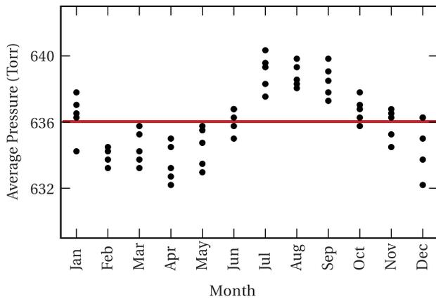
FIG. 6. Monthly averaged absolute barometric pressure at our location. This 5-yr data set shows that the annual pressure variation is approximately 5 Torr, on average. This pressure change, if not controlled, could produce annual fractional changes in the  $\beta$  count rate of up to 0.0015, depending on the sample being measured.
