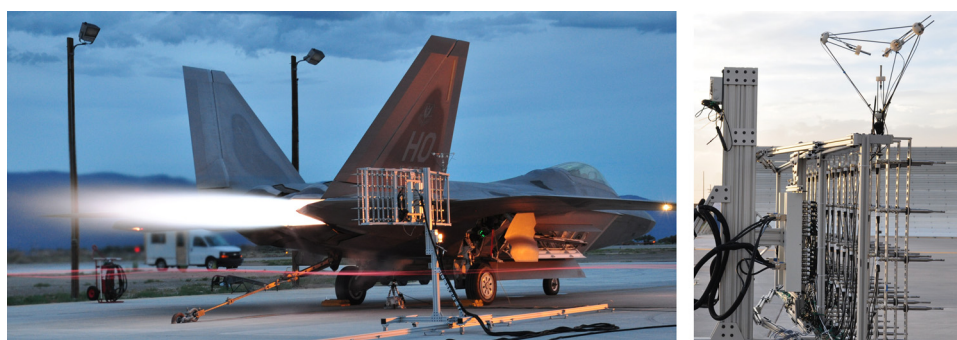
Fig. 1. (Color online) Measurement setup with static engine firing (left), and close-up of microphone rig and intensity probe (right). The rig and probe were mounted to an aluminum guide rail to ensure accuracy of the measurement plane geometries.
