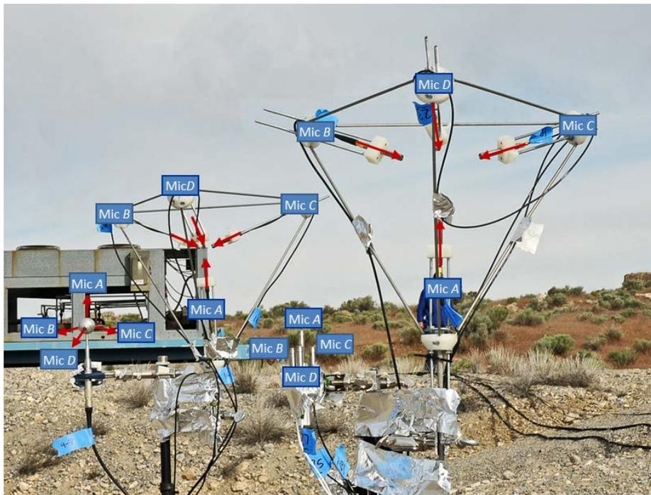
Fig. 4 - Orion-50 collocated four-probe measurement layout. Orientation of the four probes and microphones are shown with the plume coming out of the page.
