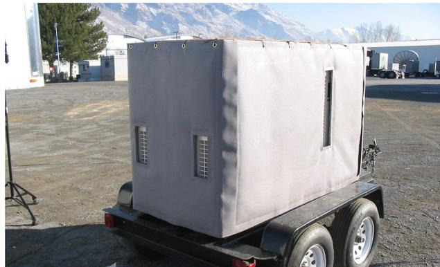
**Figure 3.** Transmission loss pads applied to the genset. The pads were custom made to fit the vent openings in the panels.
