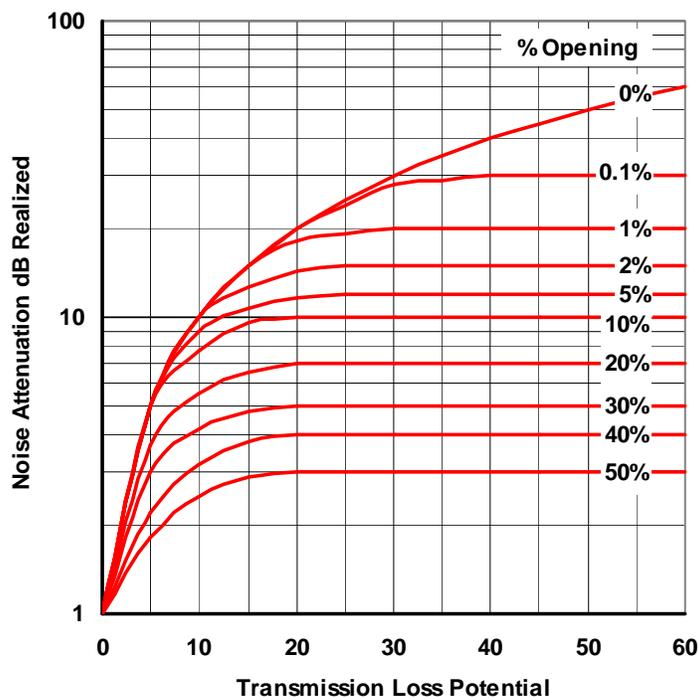
**Figure 1.** Chart of possible noise attenuation realized as a function of the original transmission loss potential and the percent open area of the enclosure (adapted from Bell<sup>3</sup>).
