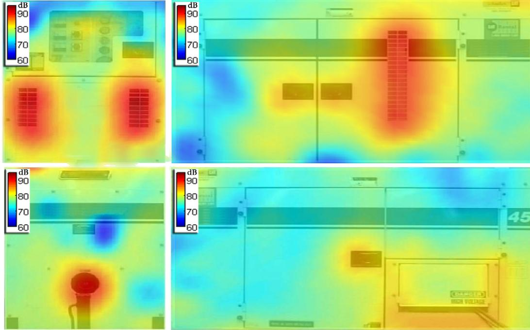
**Figure 2.** Nearfield intensity scans of each side of the genset: a) back, b) left side, c) front, d) right side (dB re:  $10^{-12}$  W).
