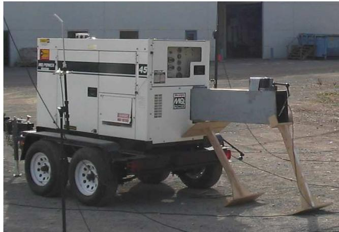
**Figure 4.** Photograph of the experimental ANC duct, located over one of the two vent openings on the back side of the genset.
