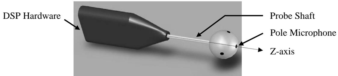
Figure 1: Energy Density Probe
