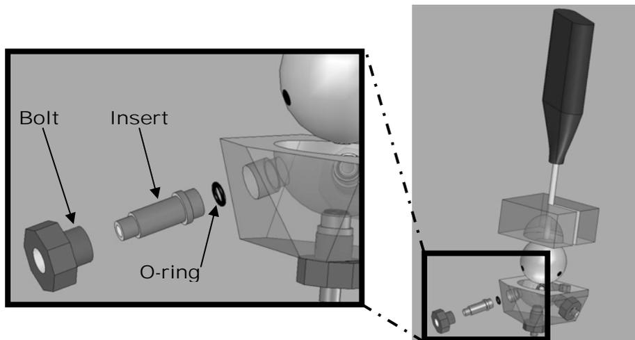
**Figure 10: CAD Model of Attachment**
