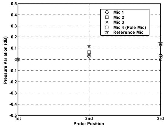
**Figure 13: Calibration Error at 250 Hz and 114 dB**
