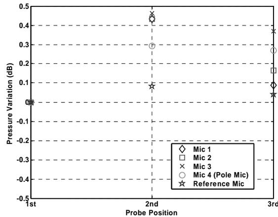
**Figure 16: Calibration Error at 2000 Hz and 110 dB**
