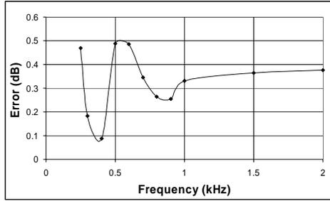
**Figure 9: Frequency Sweep of Acoustic Masses (PVC Tubes)**
