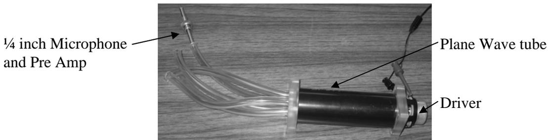
Figure 8: PVC Tube Test Setup
