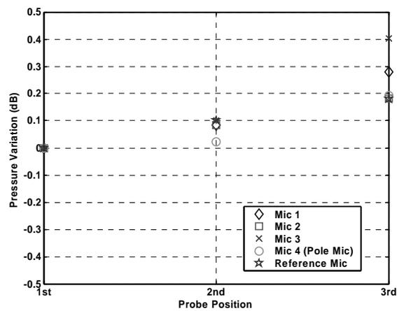
**Figure 15: Calibration Error at 1000 Hz and 114 dB**
