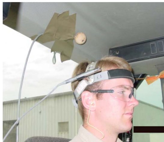
Figure 1: (a) Wheel loader used in this study. All tests were performed with the machine stationary. (b) Sensor mounted above the operator's head.
