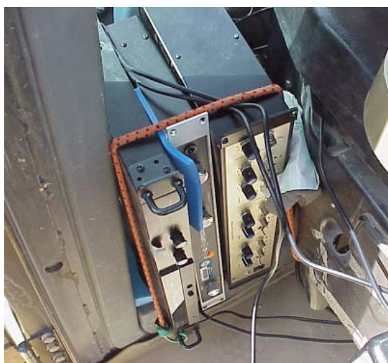
Figure 2: (a) Amplifiers and signal conditioners shown mounted on the right side of the cab. Computers and other supporting hardware were situated on the left side (not shown). (b) Consumer-quality speaker. Another speaker was mounted in a similar location on the other side of the cab.
