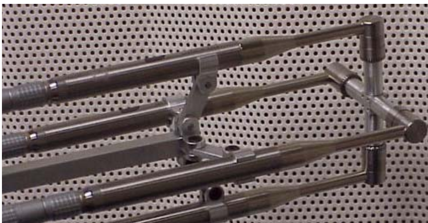
Figure 2: 2-dimensional intensity probe.
