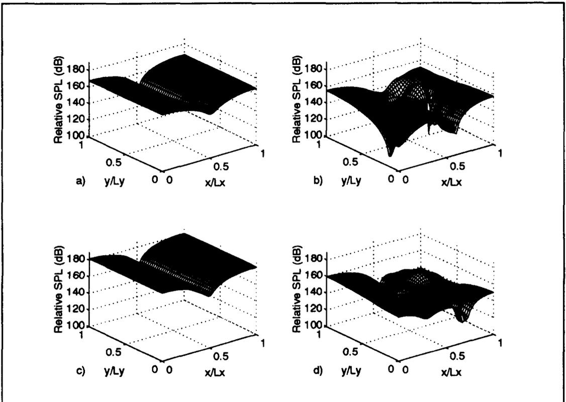
**Figure 4.** Relative sound pressure level in the  $z = 1.0$  m plane: a) No control; b) Potential energy minimized; c) Squared pressure minimized; d) Energy density minimized.
