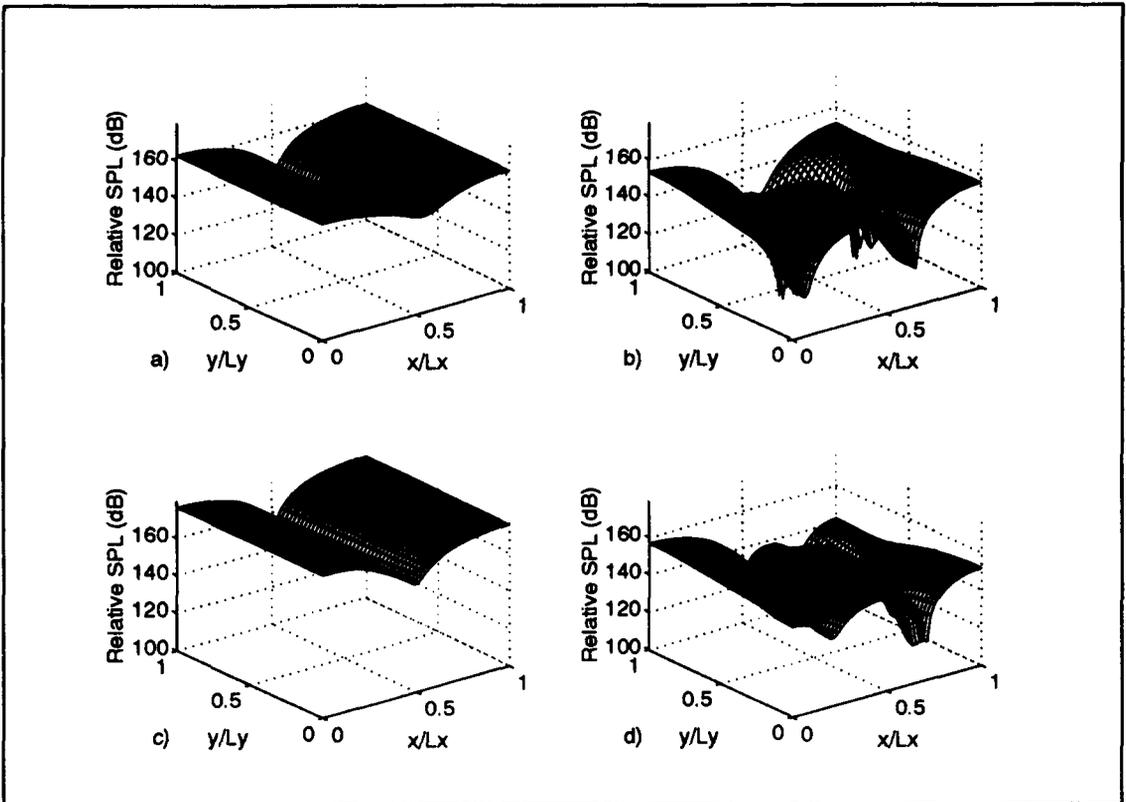
**Figure 3.** Relative sound pressure level in the  $z = 0.8$  m plane: a) No control; b) Potential energy minimized; c) Squared pressure minimized; d) Energy density minimized.
