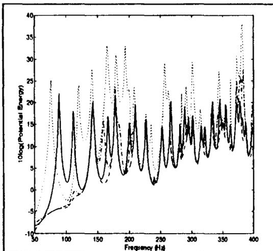
Figure 1. Potential energy in the enclosure. \_\_\_\_\_ no control; \_\_\_\_\_ potential energy; . . . . squared pressure; - - - energy density.
