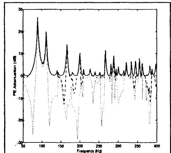
Figure 2. Attenuation of potential energy in the enclosure. \_\_\_\_\_ potential energy; . . . . squared pressure; - - energy density.
