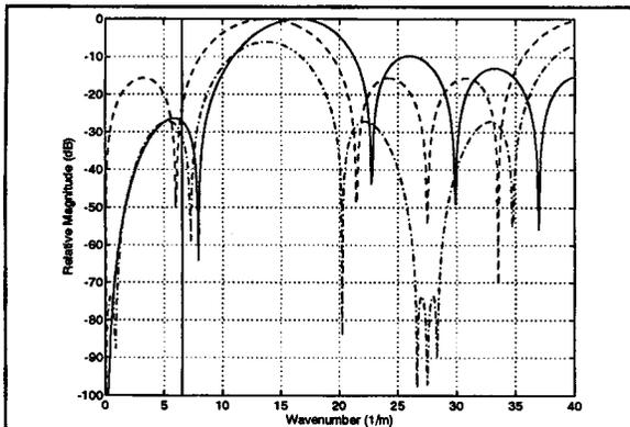
**Figure 4.** Wavenumber spectrum of beam excited in its fourth mode: \_\_\_\_\_ analytic transform; \_ \_ \_ \_ point sensors; \_ . . . distributed sensors.
