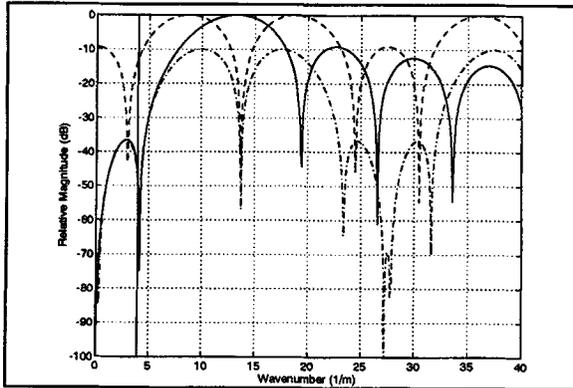
**Figure 3.** Wavenumber transform of beam excited in its third mode: \_\_\_\_\_ analytic transform; \_ \_ \_ \_ point sensors; \_ . . . distributed sensors.
