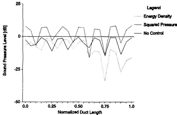
Figure 7: Measured SPL at 180 Hz with the control at  $x/L=0.69$  and error sensor at  $x/L=0.43$
