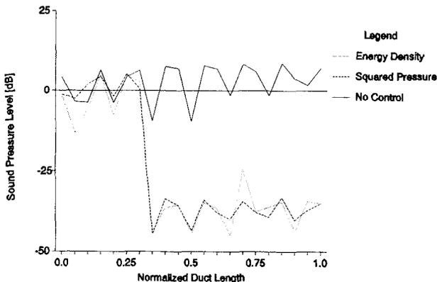
Figure 5: Measured SPL at 213 Hz with the control at  $x/l=0.34$  and error sensor at  $x/L=0.47$ .
