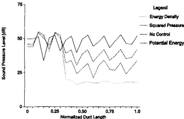
Figure 3: Predicted SPL at 200 Hz with the control at  $x/L=0.34$  and error sensor at a  $x/L=0.47$ .
