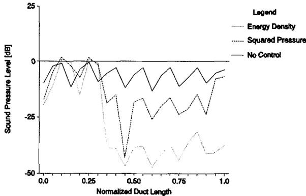
Figure 6: Measured SPL at 200 Hz for the control at  $x/L=0.34$  and error sensor at  $x/L=0.47$ .
