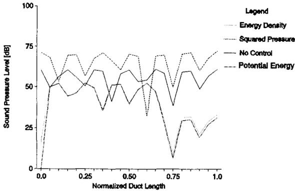
Figure 4: Predicted SPL at 180 Hz with the control at  $x/L=0.69$  and error sensor at  $x/L=0.43$ .
