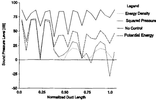
Figure 2: Predicted SPL at 213 Hz with the control at  $x/L=0.34$  and error sensor at  $x/L=0.47$ .
