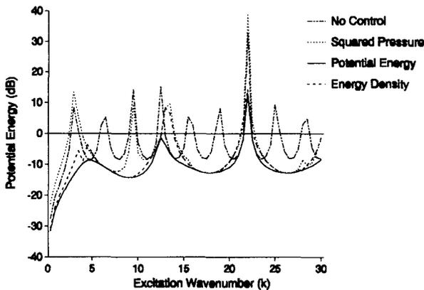
Figure 2. Total potential energy in the duct. For the squared pressure and energy density, the discrete sensor is located at the position  $x = 0.5L$ .
