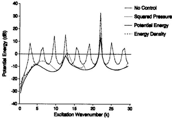
Figure 5. Total potential energy using multiple sensors. Squared pressure sensor locations:  $x = 0.02, 0.1, 0.2, 0.3, 0.4, 0.5, 0.75, 0.98L$ . Energy density sensor locations:  $x = 0.5, 0.98L$ .
