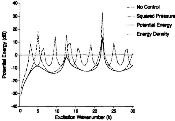
Figure 1. Total potential energy in the duct. For the squared pressure and energy density, the discrete sensor is located at the position  $x = 0.98L$ .
