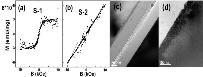
**FIGURE 1.** The magnetization vs. the applied magnetic field measured at 10 K for (a) S-1, and (b) S-2. TEM micrograph of sample S-1 (c) near the amorphous-crystalline boundary region, (d) higher magnification image at the a-c interface.
