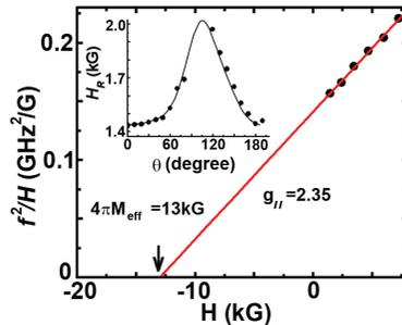
**FIGURE 2.** Frequency dependence of the FMR resonance peak with the magnetic field applied in the plane of the substrate surface. The inset shows the resonance field  $H_R$  as a function of the angle between the B field and the plane of the substrate.
