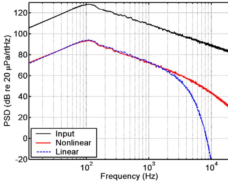
**Figure 4:** Power spectral density (PSD) of the input shaped random noise at 10 m and the linearly- and nonlinearly-predicted spectral densities at 500 m. The linear prediction exceeds -200 dB re 20 μPa/√Hz at 20 kHz.
