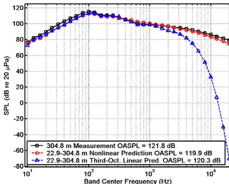
**Figure 1:** Measured and predicted third-octave spectra at 304.8 m and one engine at afterburner.
