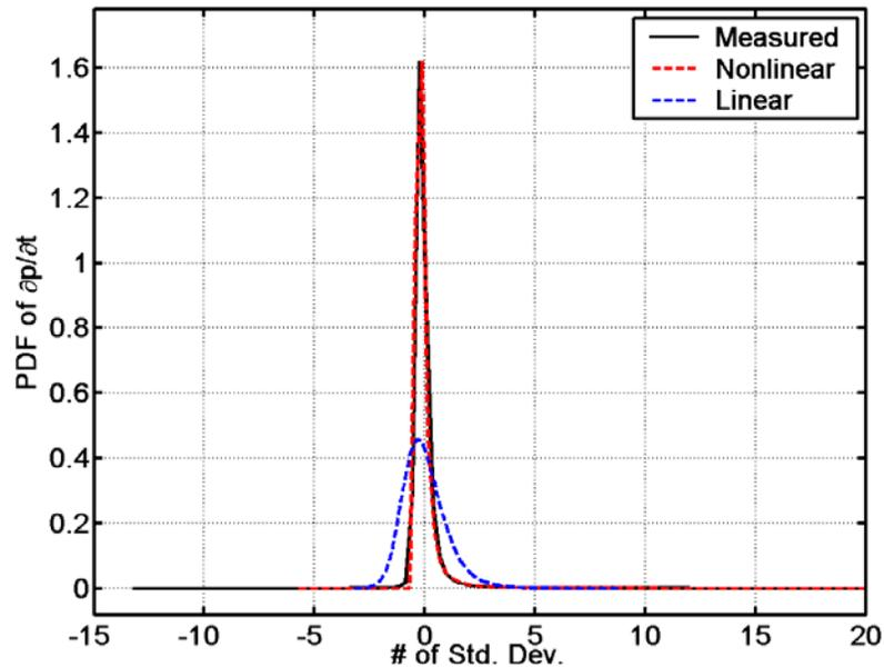
**Figure 3:** Probability density functions of the 304.8-m AB waveform time derivatives. The positive tails for both the measured and nonlinearly-predicted distributions extend out to approximately 63 standard deviations.
