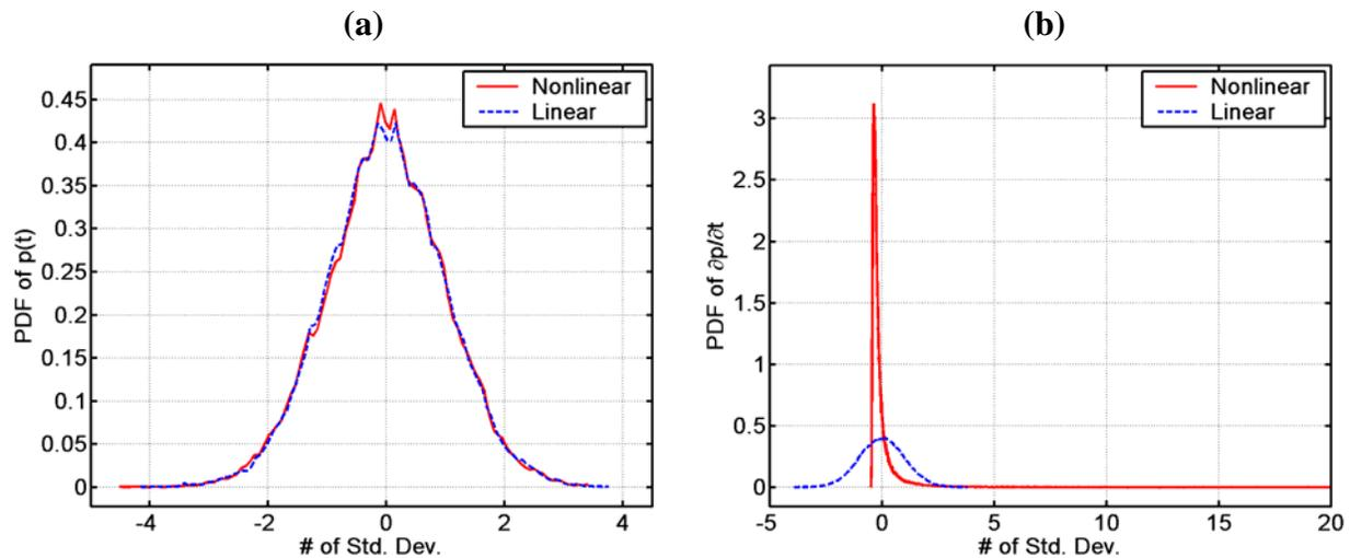
**Figure 6:** Probability density functions of the (a) waveforms and (b) waveform time derivatives at 500 m. Positive derivative values for the nonlinearly-propagated waveform continue out to nearly 79 standard deviations.
