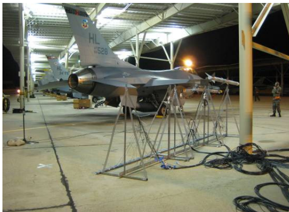
Figure 5: Array with microphones 1.5" off the ground, left; Measurement chassis, hard drive, and laptop showing LabVIEW-based data acquisition code, on right.
