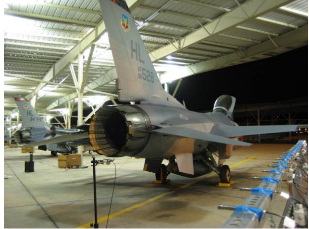
Figure 3: Microphone array with microphones 5 ft off ground, left; reference microphone on tripod in front of array, on right.
