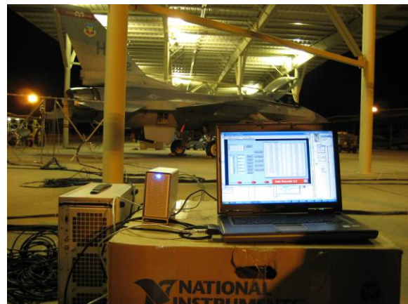
Figure 5: Array with microphones 1.5" off the ground, left; Measurement chassis, hard drive, and laptop showing LabVIEW-based data acquisition code, on right.
