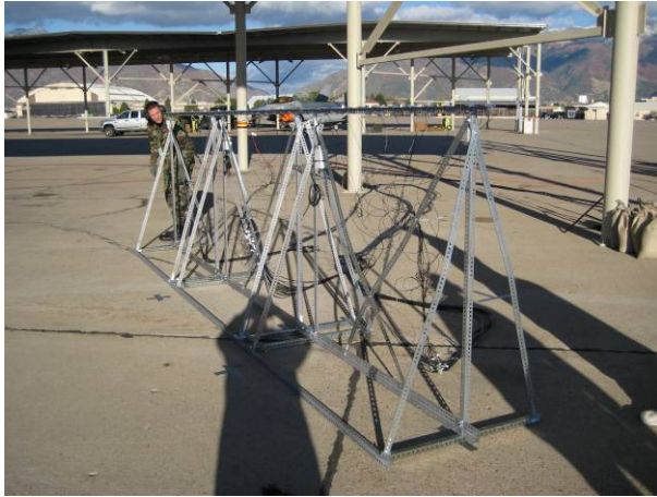
Figure 3: Microphone array with microphones 5 ft off ground, left; reference microphone on tripod in front of array, on right.
