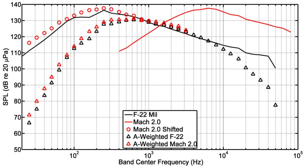
Fig. 7 – One-third octave band spectra of the F-22A at military conditions (black) and the Mach 2.0 laboratory jet (red) at locations of peak radiation (see arrows in Fig. 2), with amplitude scaled upward by 6 dB. The peak-shifted laboratory spectrum is represented with circles, and the A-weighted spectra are represented with triangles.
