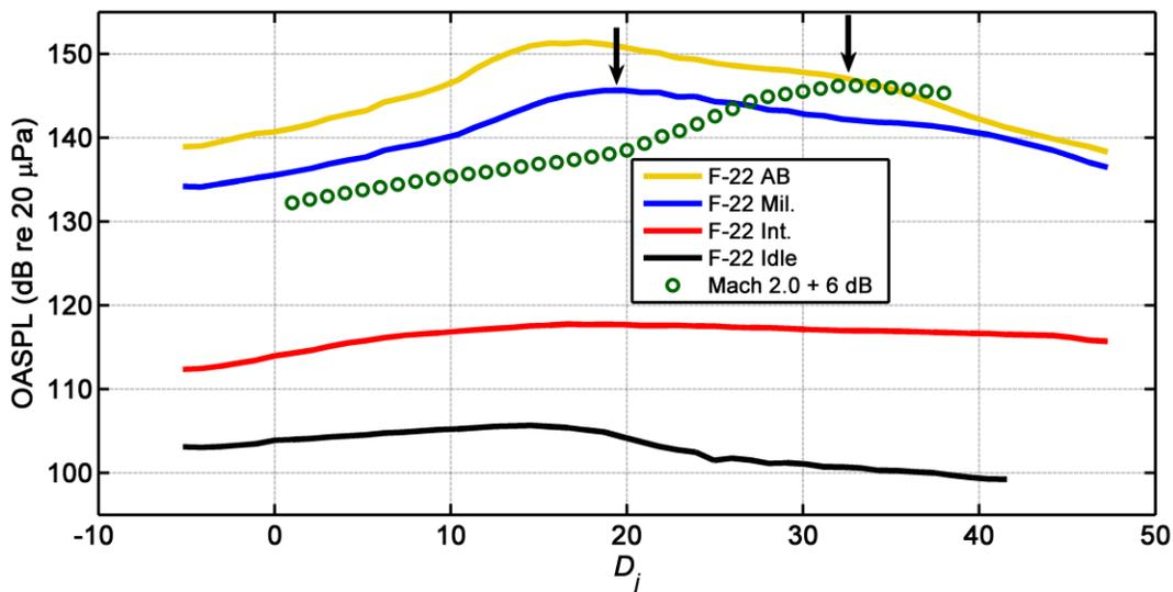
Fig. 2 – Unweighted OASPLs for all engine conditions of the F-22, recorded along the ground-based microphone array, as a function of distance downstream in nozzle diameters  $D_j$ . The circles indicate the unheated, Mach 2.0 laboratory data (described in Section 3) adjusted by 6 dB to account for the absence of ground reflections in the anechoic chamber. The arrows indicate the maximum OASPLs for the laboratory jet and the F-22A at military power.
