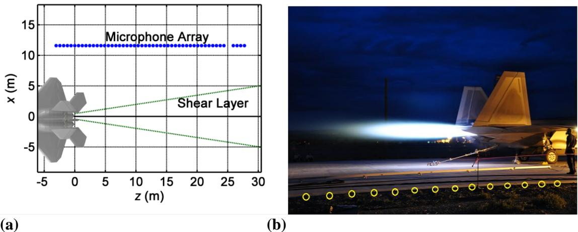
Fig. 1 – Placement of ground-based microphones during the F-22A experiment 11.7 m from the jet centerline. Microphones for this experiment are represented by the blue dots parallel to the centerline of the jet plume on the left and the yellow circles on the right.
