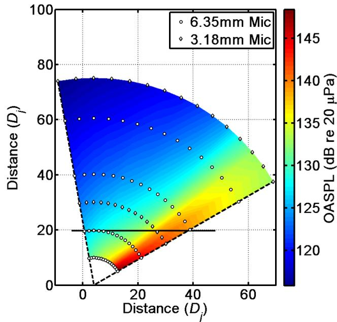
Fig. 6 – Interpolated OASPL of the ideally expanded, unheated, Mach 2.0 laboratory jet, with the nozzle at (0,0) and exhausting to the right. The white marks denote microphone locations. The equivalent scaled location of the F-22A ground-based microphone array is demarcated by the black line.
