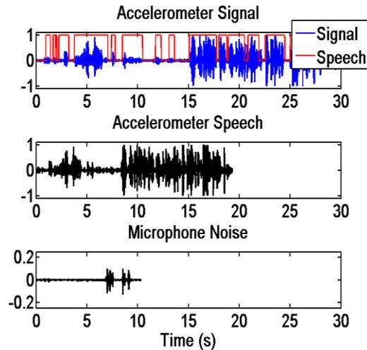
Figure 8. Separation and splicing of speech and noise using the accelerometer.
