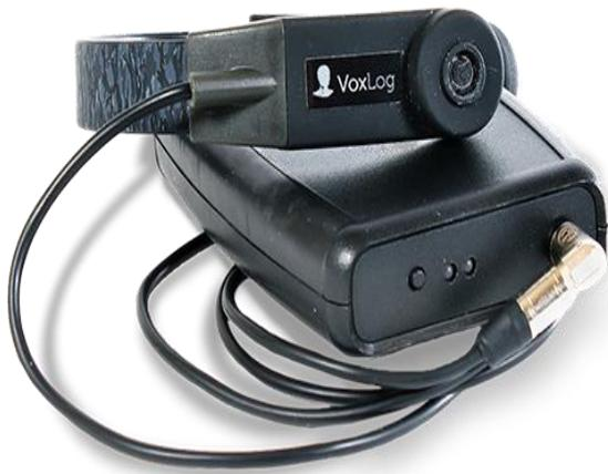
Figure 7. Sonvox VoxLog collar with accelerometer and microphone.
