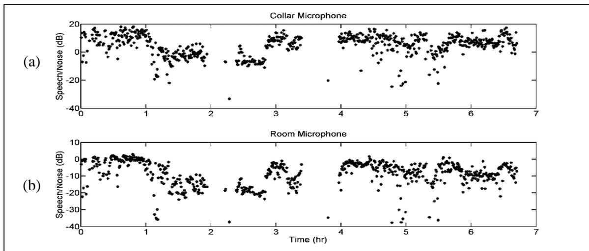
Figure 9. Examples of speech-to-noise levels over time. Plot (a) shows speech-to-noise levels calculated using the collar microphone. Plot (b) shows speech-to-noise levels calculated using the room microphones.
