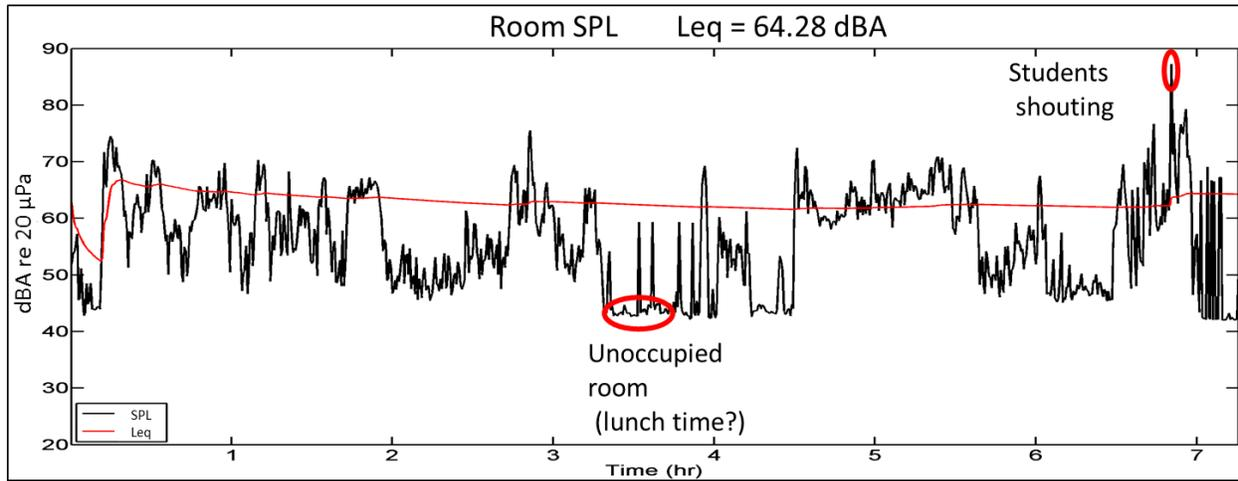
Figure 6. Time-dependent noise levels in one of the classrooms over time.
