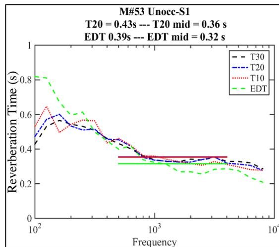
**Figure 4. Reverberation time in one of the measured classrooms. The reverberation times at mid frequencies were of special interest, because of their importance for speech.**
