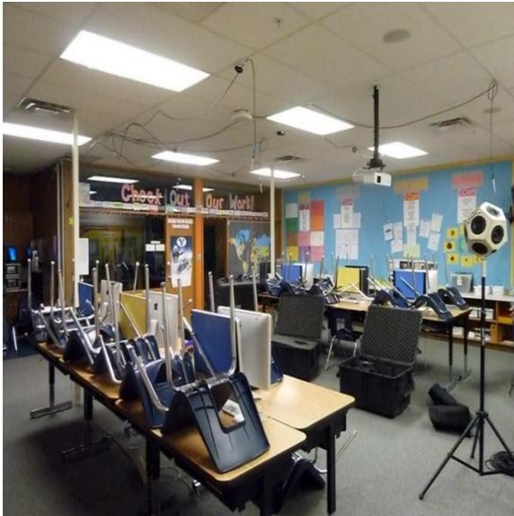
**Figure 1.** Microphones were hung from the ceiling in each of the classrooms. Also pictured is a dodecahedron loudspeaker used in the impulse response measurements.
