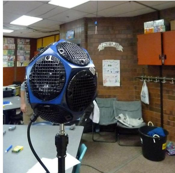
**Figure 2.** Another dodecahedron loudspeaker used in impulse response measurements in the classrooms.
