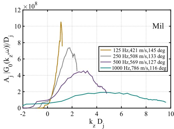
**Figure 8** Frequency-dependent wavenumber spectra at military power. Scaled, data-educed, axial wavenumber spectra as a function of frequency for the tethered F-22 with a single engine operated at military power. The estimated convective speed and corresponding angles are relative to the reference point  $z = 5.5$  m from the nozzle exit plane, as illustrated in Figure 4.
