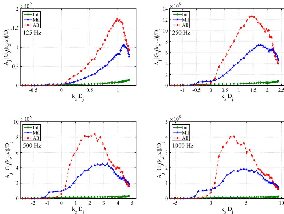
**Figure 7.** Scaled, data-educed, axial wavenumber spectra for 125, 250, 500, and 1000 Hz. The wavenumber spectra are obtained using the LSS spectral decomposition of the aircraft noise measured of 50 ground-based microphones when one engine was operated at intermediate (green), military (blue), and afterburner (red) power.
