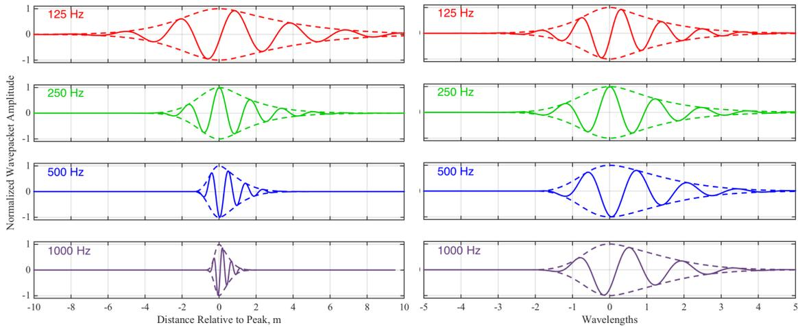
**Figure 10** Optimized wavepackets at 125, 250, 500, and 1000 Hz. (Left) The real part and magnitude of normalized axial wavepackets for the modeling parameters that yield the best agreement with the data-educed wavenumber spectra from the F-22, with one engine operated at military power, plotted as a function of distance in meters. (Right) The same wavepackets plotted as a function of acoustic wavelength.
