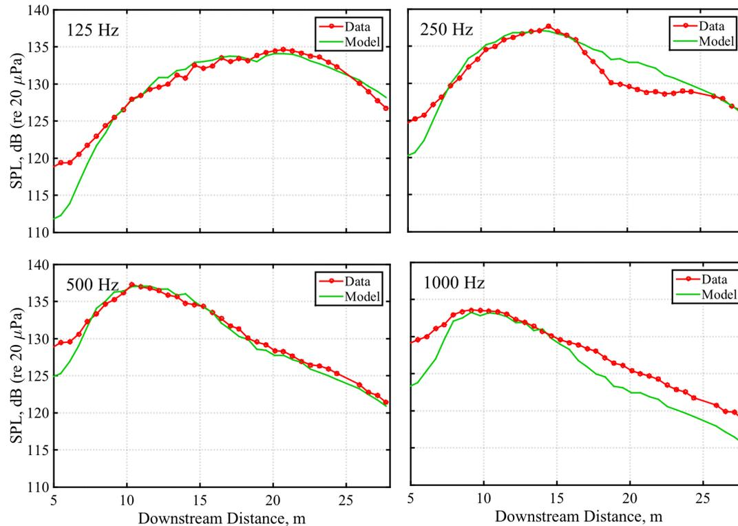
**Figure 11 Comparison of measured and predicted levels.** The levels predicted by the equivalent wavepacket model (solid) are compared to levels measured on the ground-based microphones (dotted), at military power. The modeled levels are based on the optimized wavenumber spectra and the amplitude is shifted to match the peak level.
