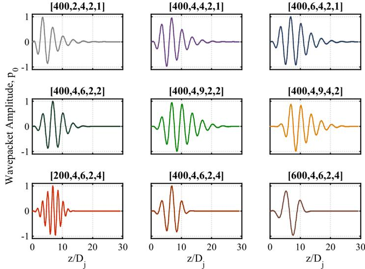
**Figure 1. Wavepacket shapes.** *Examples of the real parts of the axial wavepacket shapes at 250 Hz for the parameters listed above each plot:  $[U_c, b_1, b_2, g_1, g_2]$ .*
