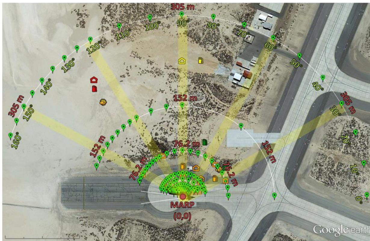
**Figure 1. Measurement locations near Pad 18 at Edwards Air Force Base.** Various arrays and arcs of microphones were located around the aircraft, including two cranes not pictured at 610 and 1220 m along the  $135^\circ$  radial, which featured microphones 9.14 m above the ground.
