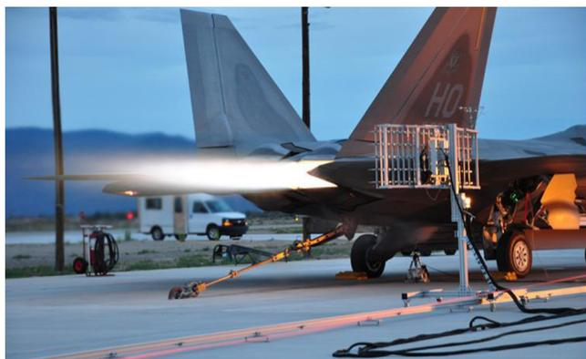
Fig. 2—The tied-down F22A Raptor with one engine at afterburner. Shown also is the 90-microphone rectangular array.
