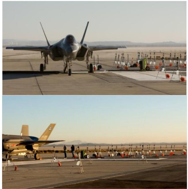
Fig. 1—Tied-down F-35 AA-1 aircraft, with a portion of the geometric near-field microphone array.
